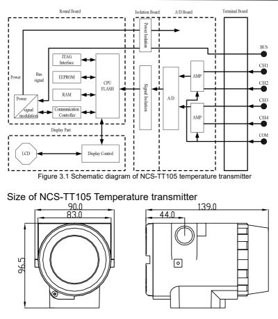
Figure 3.2 Size of NCS-TT105 temperature transmitter (unit: mm)
