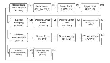
Figure 7.4 Adjusting Function and LCD Display
