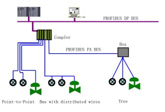
Figure 5.1 PRFIBUS PA network topology
