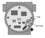
Figure 6.5 HART smart transmitter hardware jumper
