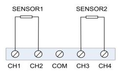
Figure 2.7 Wiring of NCS-TT105 temperature transmitter(2-wire)
