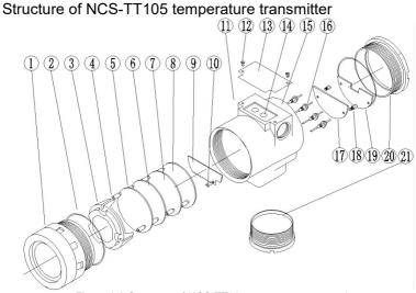
Figure 3.3 Structure of NCS-TT105 temperature transmitter
