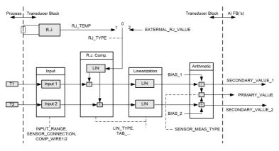
Figure 5.3 Transducer block structure
