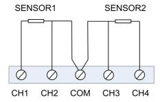
Figure 2.6 Wiring of NCS-TT105 temperature transmitter(3-wire)
