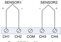
Figure 2.8 Wiring of thermocouple
