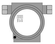
Figure 4.7 NCS-TT105 temperature transmitter hardware jumpers
