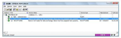
Figure 5.9 Scan DP bus and List PA device
