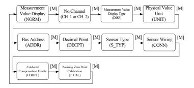
Figure 7.3 Adjusting Function and Display
